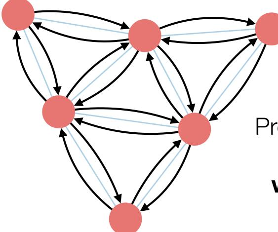
Propagate features from each node to adjacent nodes, weighted by edge score
