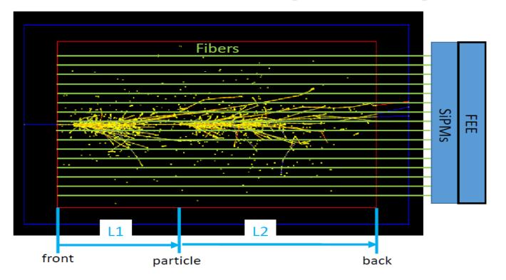
Signal Time = L1/c + L2/kc, c = velocity of particle kc = velocity of light in fiber (k $^{\sim}$ 0.6)  $\Delta$ L = 2 cm = 44 ps
