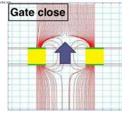
The electron transparency has been determined with different measurements and corresponds to 82 % as expected from simulations.
