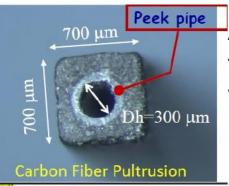
Alternatively, Lund is exploring micro channel cooling together with Pisa. These consists of pipes with Ø 300 µm in carbon fiber tubes.
