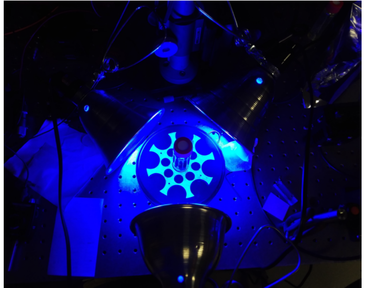
450 nm curing station. Sample is rotated 1.2 rpm during curing
