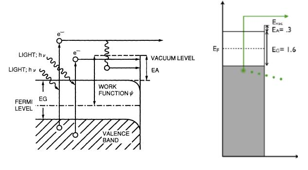
Left: Schematic of the Energetics for alkali photocathode vacuum emission – the pair energy Ea+Eg is near the vacuum level.
