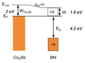
*L*: Energy bands  $Cs_3Sb$ , BN. *R*: Implied electrostatic potential *lowers* Ep from 2 eV  $\rightarrow$  1.6 eV
