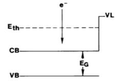
VB=Valence Band, CB=Conduction Band, VL=Vacuum Level,  $E_G$ =Band Gap,  $E_{th}$  is Ep, the threshold energy to produce electron-hole pairs.
