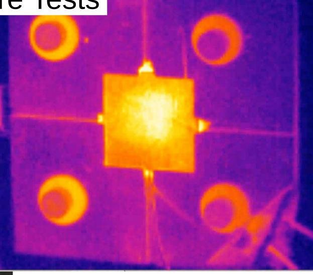
LiF is deposited on a Ta backing plate.
