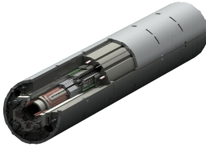
Figure 4: MQXFA 3-D conceptual cutaway view
