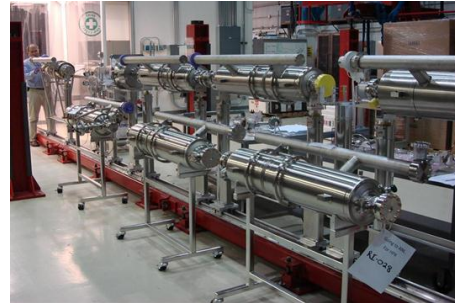
Cavity string assembly rail inside Fermilab's Cryomodule Assembly Building.
