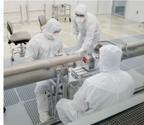
Technicians connecting superconducting cavities together in Fermilab's clean room
