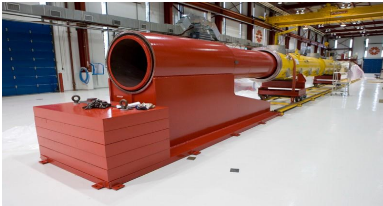
Fixtures in ICB were used to assemble a 1.3 GHz cryomodule
