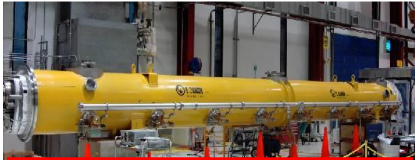
1 st U.S. built ILC/PX Cryomodule
