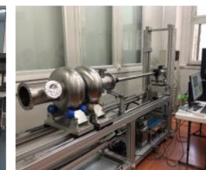
Cavity inspection camera and grinder
