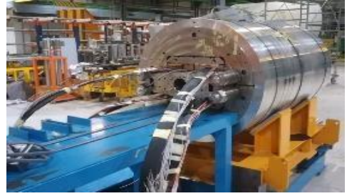
2018: FRESCA2 (100 mm aperture, 14.6/14.95 T bore/peak at 12.1 kA, 1.9 K)
