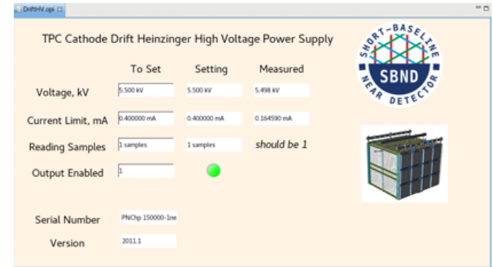
Interface for HV power supply
