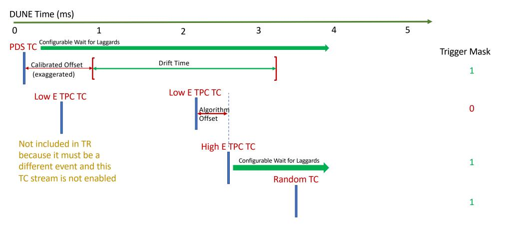
Trigger Record would record that 4 TCs were in coincidence, because random's time window would include prior event data
