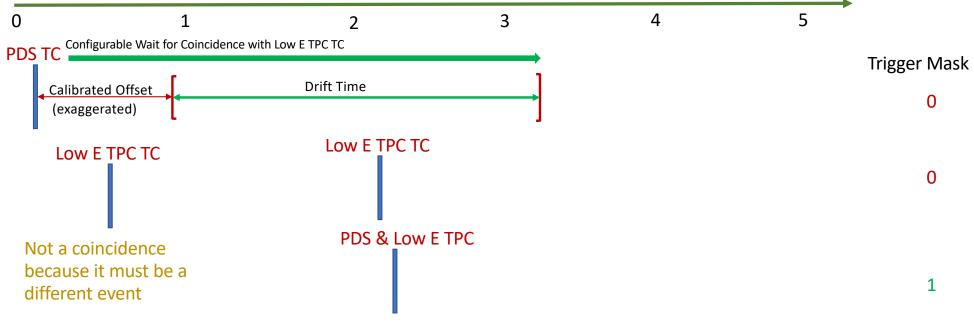
Trigger Record would still record that a PDS & LE TPC satisfied coincidence trigger; record bits and coincidence bit
