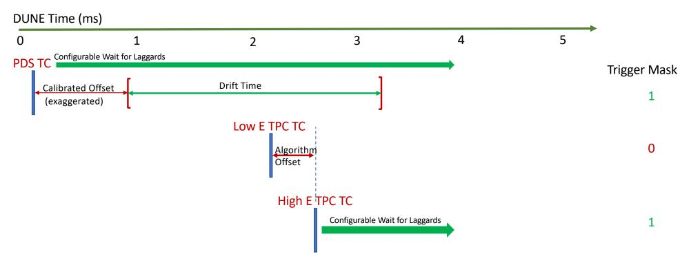
Trigger Record would record that 3 TCs were in coincidence, even though one here (LE) could not have created a TD on its own Coincidence is not <u>required</u> here for a TD; it just happens to occur
