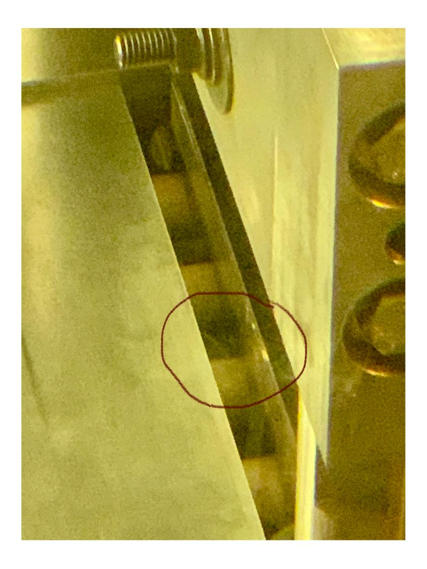
This is the washer we recovered from the Stripline block. Note the blister caused by electric current.
