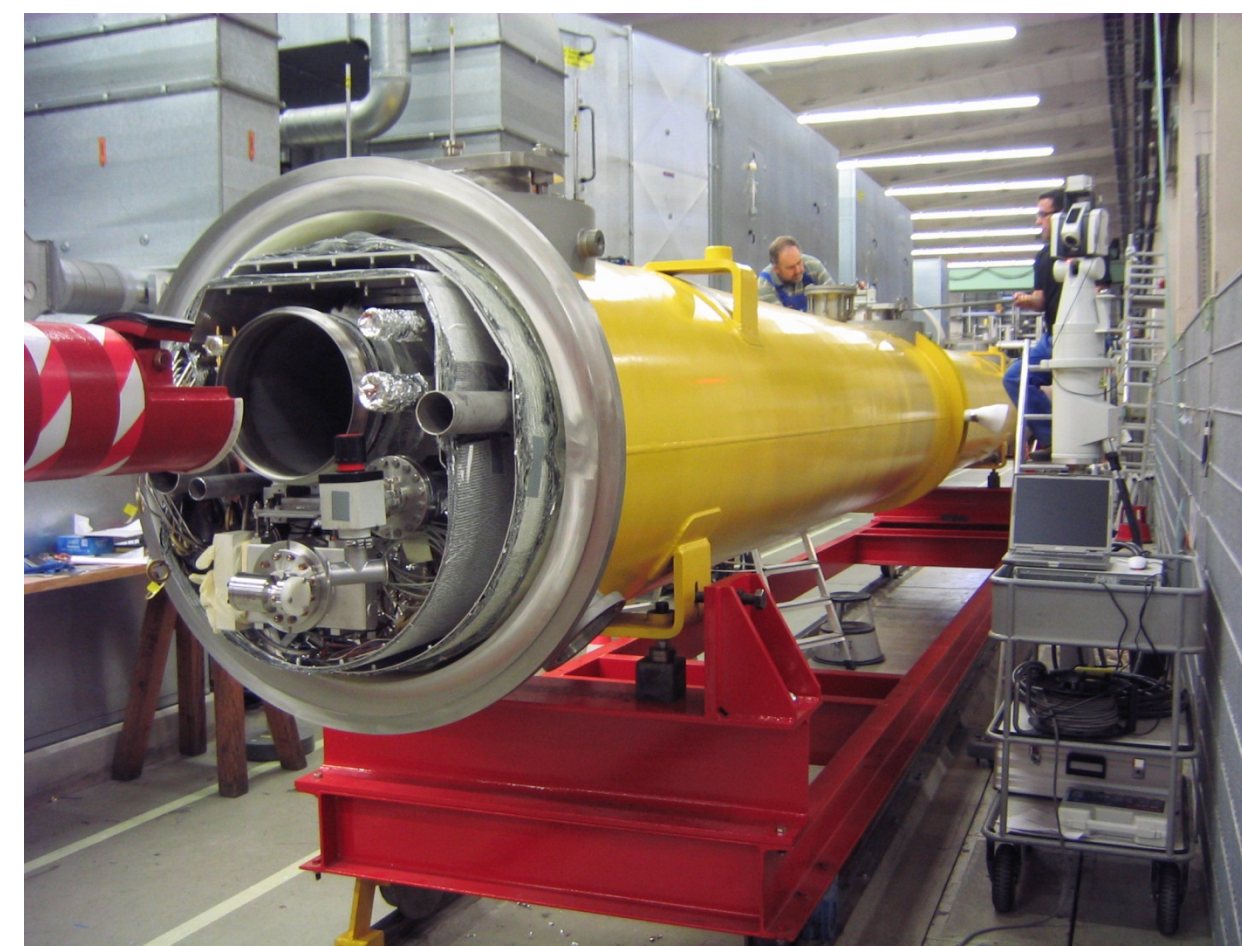
Aligning the cold mass into the vessel
