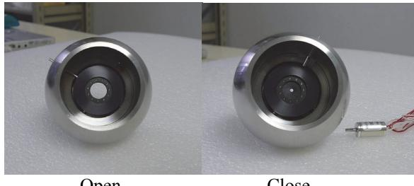
Fig.14 Iris diaphragm target, four targets will be used simultaneously. The diaphragm in measurement is close to form a small circle of iris, and other three are open.
