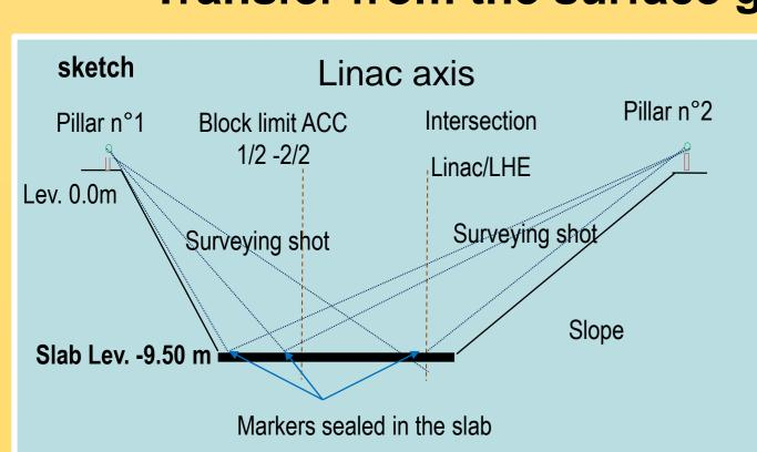
The axes of the beam lines (Linac and LHE) were indicated on the concrete slab at level -9.50 m from pillars 1 to 4 of the surface geodetic network. This operation was carried out before the concrete slabs of the higher levels were cast.
