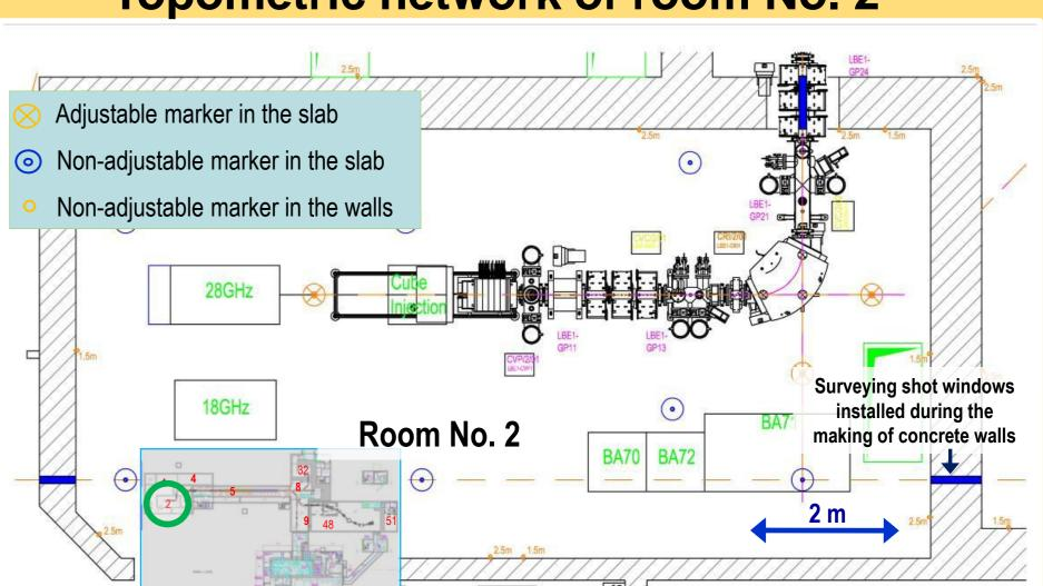
The room and process topometric network started in July. Measurement of the topometric network is made more complicated by the walls between the various rooms. Surveying shot windows were planned between the rooms during the building programming studies.
