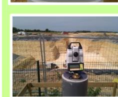
Measurement of the geodetic network
