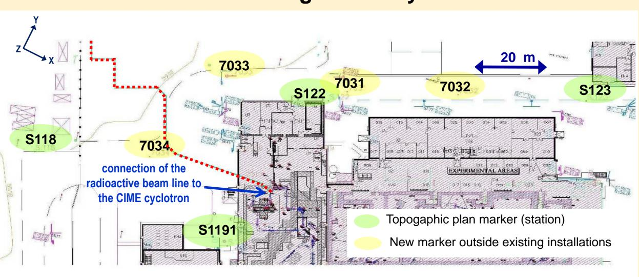
Connection of the local geodetic system to the national system around the GANIL facility
