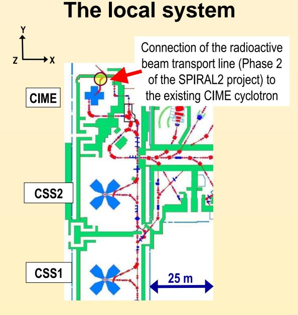
The GANIL local system is a coordinate Cartesian system defined by the centres of the two cyclotrons; CSS1 and CSS2. These centres are represented by plates concrete foundations supporting the cyclotrons at level -1 of the accelerator building.
