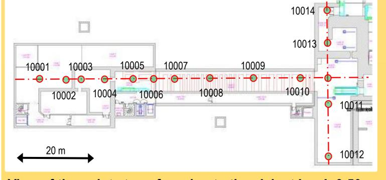
View of the points transferred onto the slab at level -9.50 m Base of the building and process topometric network
