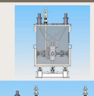
•Cold mass (cavity string, tuners) supported from strongback
