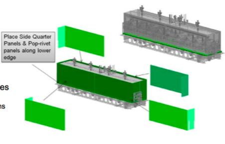
µ-metal shield required less parts
