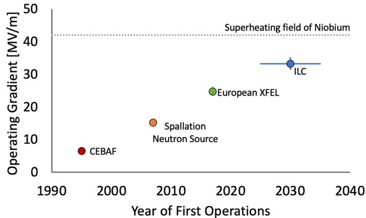
**Fig. 1:** Progress with time in SRF R&D leading to higher operating gradients for large SRF accelerators.
