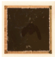
Bump Bonded VIPRAM with PRAM on top
