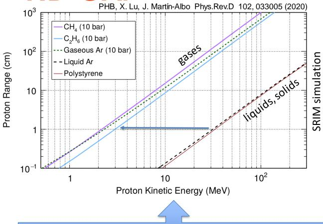
10 bar pressurized gas has ~10x lower tracking threshold, compared to liquids and solids.
