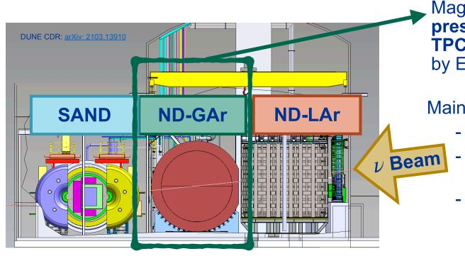
Magnetized (0.5T) high pressure gaseous argon TPC (HPgTPC) surrounded by ECAL calorimeter
