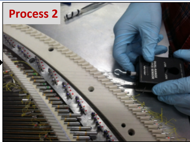
Process 2 Straw Installation (1 day)
