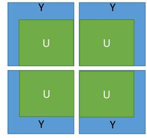
Displacing planes is not too difficult, but building readout volume would require 4 pieces put together correctly (instead of one) Not sure if there are any assumptions on ROP centering later on 14
