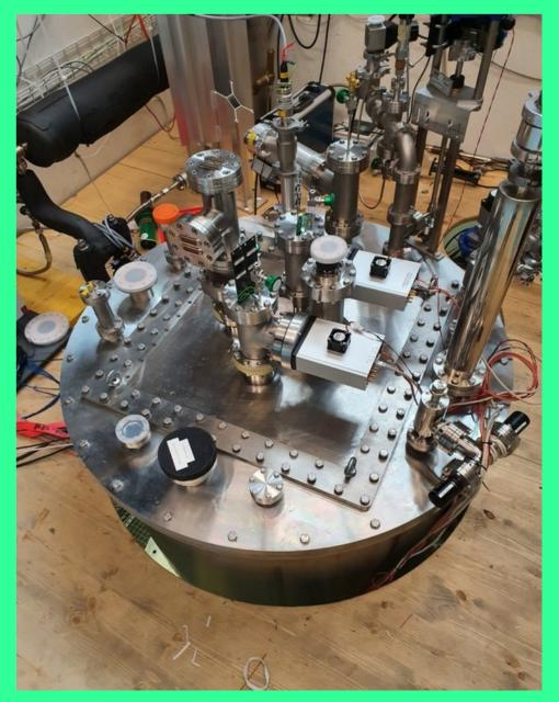
The module is installed with no difficulties Cable connectivity tests are OK Slow control 100% operative Powered LArPix tiles LArPix Hydra networks built Tests according to the LBNL program are in progress...
