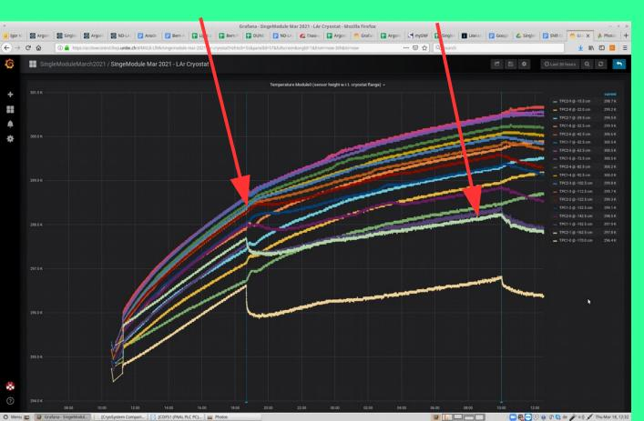
Temperatures reached max at ~27.5C and flattened.
