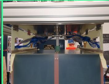
Cables are wixed with copper wire Covered with teflon tape (not tight!)
