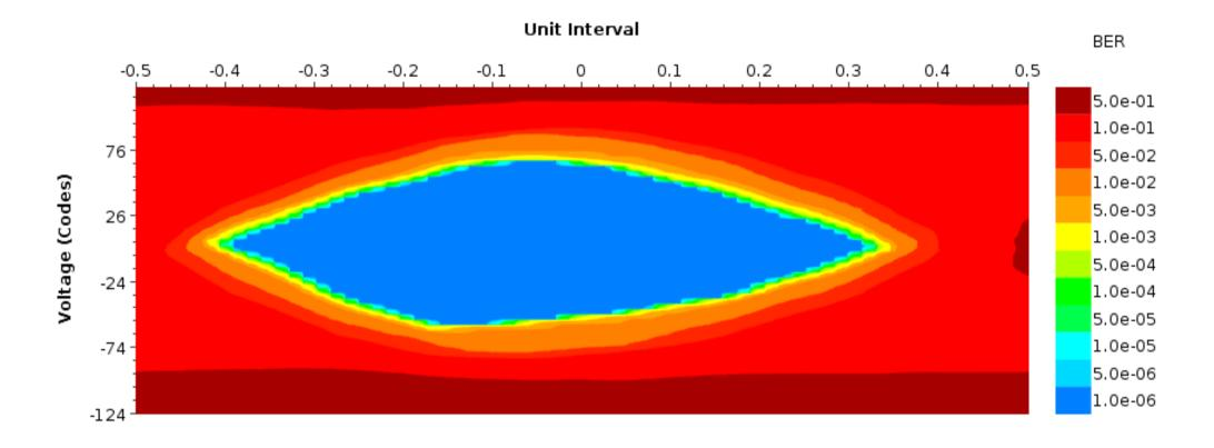
PBRS7, with 2x2x400nH inductors for power injection/extraction
