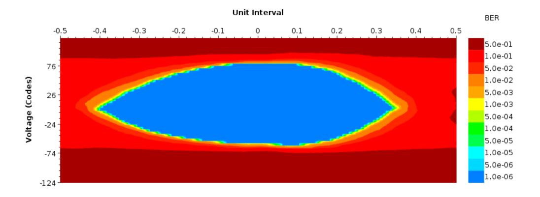
PBRS7, with 2x2x400nH inductors for power injection/extraction
