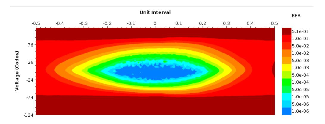
PBRS31, with 2x2x400nH inductors for power injection/extraction
