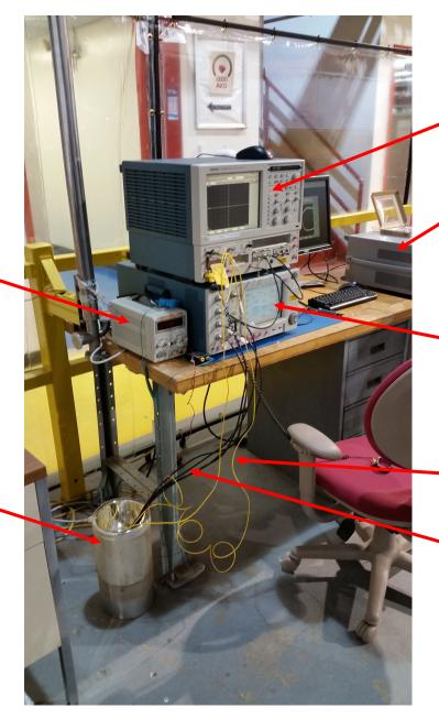
Digital Signal Analyzer (Eye pattern and jitter analysis)
