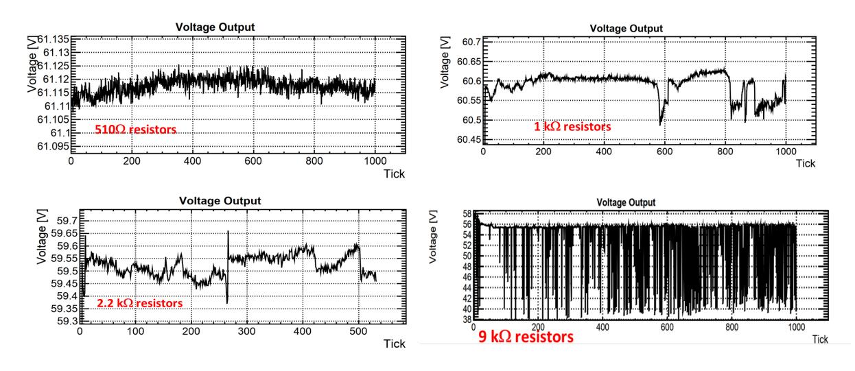
For all measurements we have seen bubbles, the higher resistors used, the more bubbles produced.
