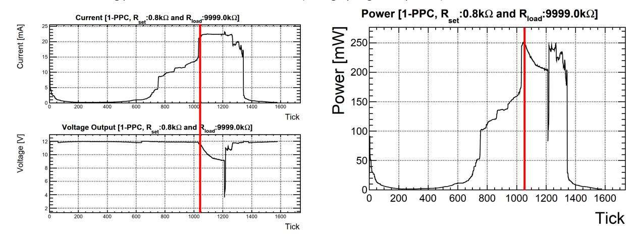
Maximum power 250 mW (11.4 V, 22 mA), load resistors is around 500 ohm
