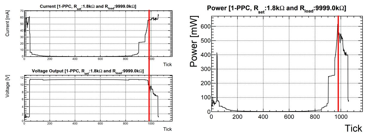
Maximum power 600 mW (11.1 V, 54.8 mA), load resistors is around 200 ohm
