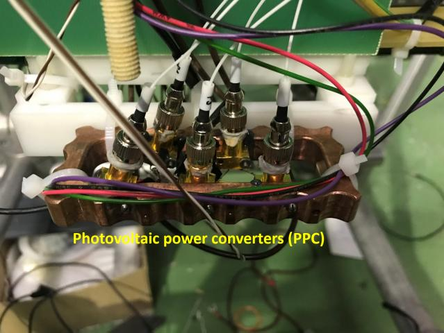
One PPC provides ~12 Volts in LAr Four in series used to get 48 Volts for SiPM arrays
