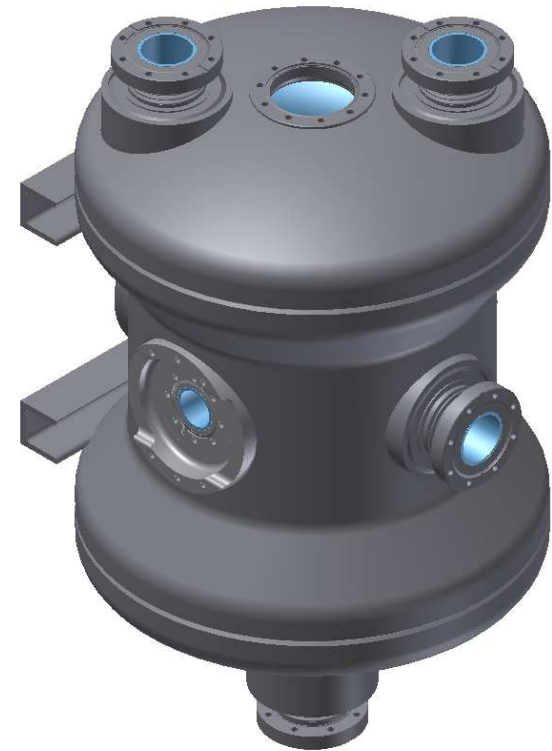
S.S. Helium Jacket S.S. Flanges Nb Cavity
