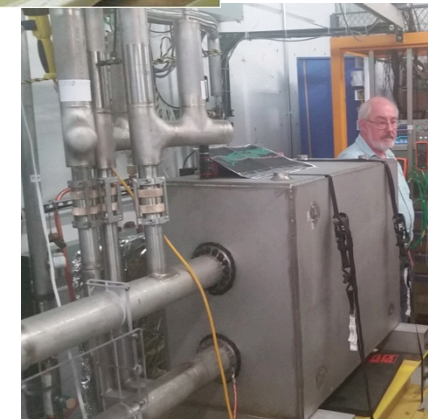
FNAL 12 T/s HTS 0.6 T max Need to push in field and speed
