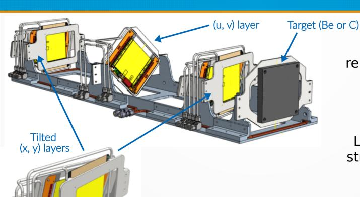
Stringent request: relative position within a station must be stable at 10 µm.
