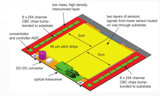
Complete and uniform angular acceptance with one module.
