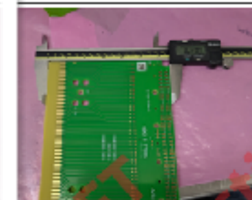
Figure 2 – Overall width measurement.
