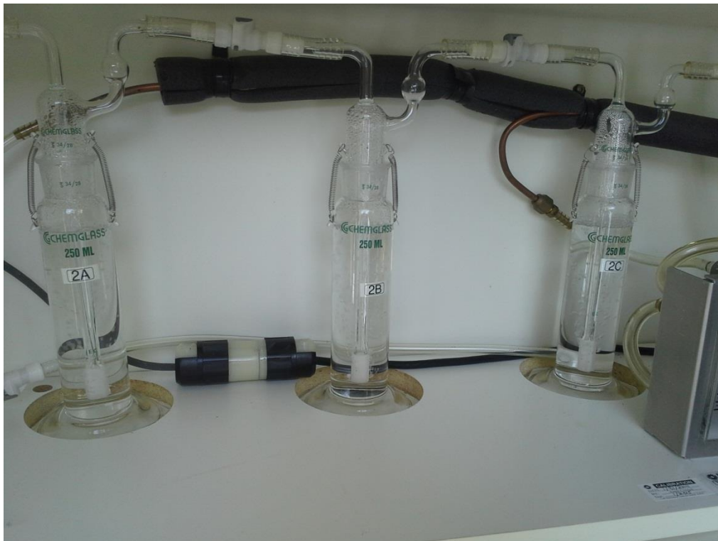
Figure F-4. Picture of the three bubblers connected in series.
