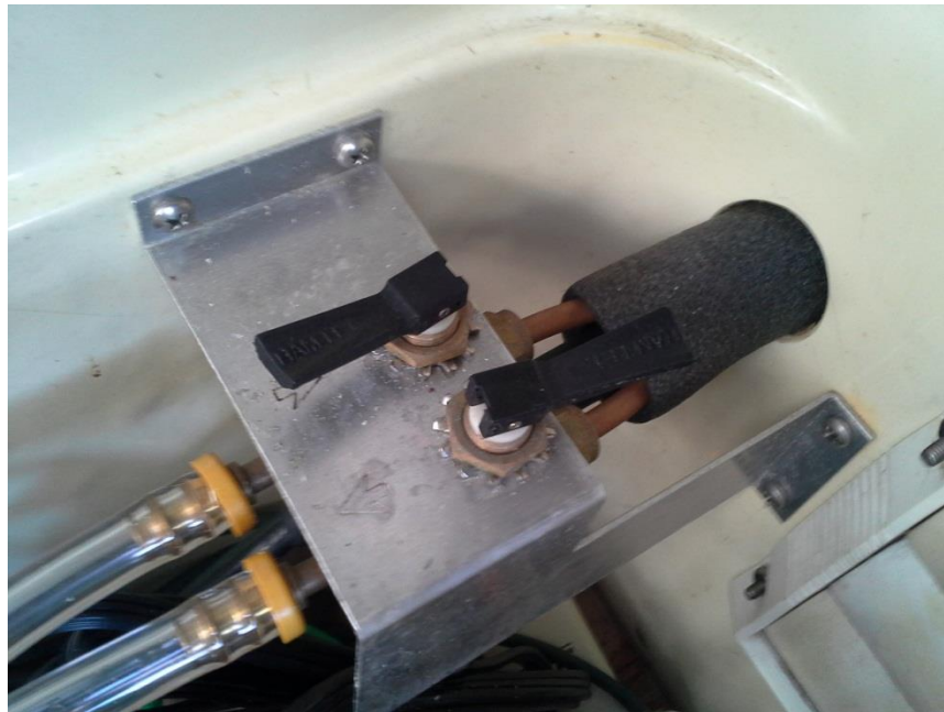
Figure F-6. Picture of the valves connecting the inlet and outlet of the sample tubes to the tritium sampler. When closed the handles are in horizontal position.
