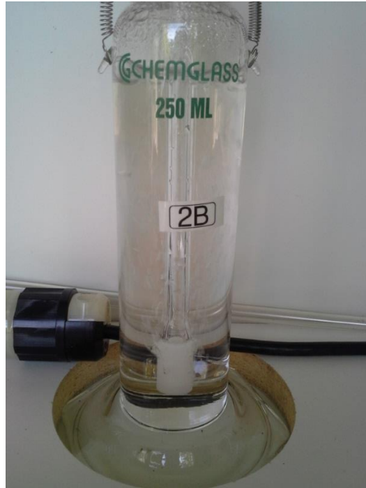
Figure F-5. Picture of a single bubbler with the two retention springs on top.
