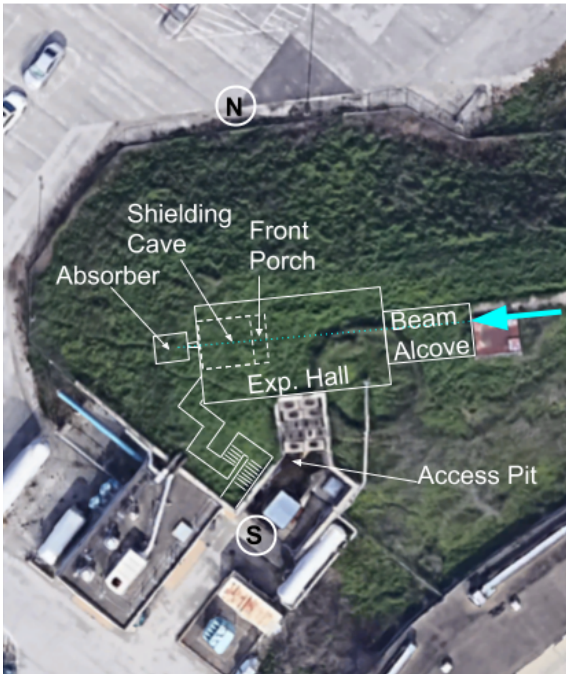
Figure 1. Annotated aerial view showing beam alcove and experiment hall approximately as situated in the grass-covered berm. Beam direction and path are indicated by the cyan arrow and dotted line. Booster Gallery West appears in the lower right corner. The points indicated by (N) and (S), directly north and south of the Front Porch position, are discussed in Sec. 3.2.2.
