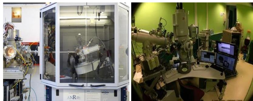
*in situ* XRD diffractometer
