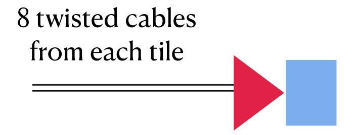
Analog Double + summing stage -> 8 twisted cables in a single OpAmp-> Analog output
