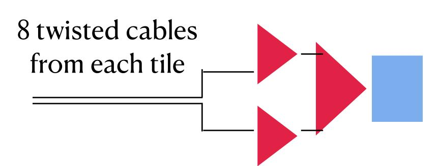
Analog Double + double summing stage -> 4 twisted cables per OpAmp + Second OpAmp to summing 4+4 -> Analog output
