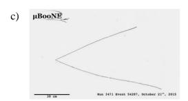
The long track is a **muon**. As minimum-ionizing particles, muons make long, straight tracks (or curve in a magnetic field), with a constant rate of energy deposition dE/dx.
