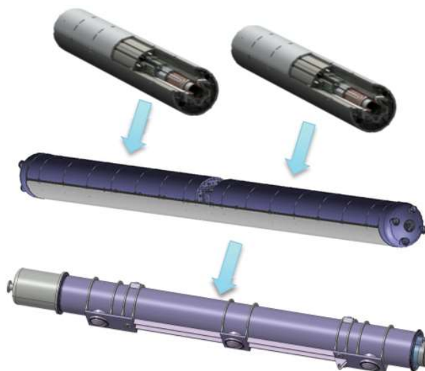
Figure 2.1: MQXFA magnets (top), cold mass (middle) and cryostat (bottom) for the Q1/Q3 elements of the HL-LHC Inner Triplet.
