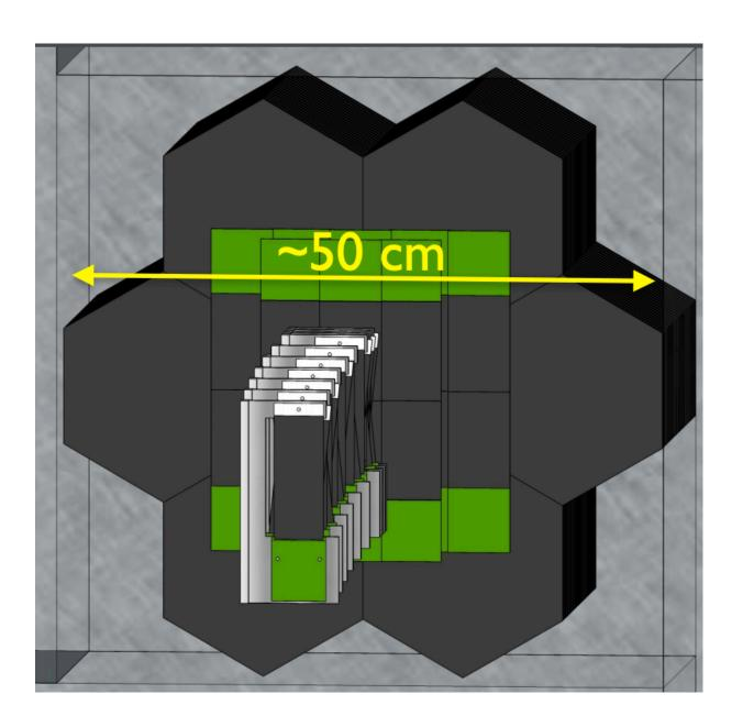
LDMX: 17 double layers of Si(-W):  $40X_{0}$  (500  $\mu$ m thick), 432 pads/module CMS (EM): 28 layers of Si(-W):  $26X_{0}$  (300  $\mu$ m thick) low and high density modules
