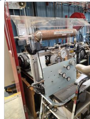
Gas injection system at PAB
