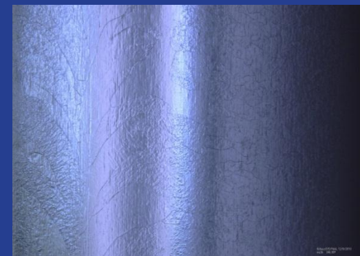
After CBP and 40 microns EP – Pit completely removed
