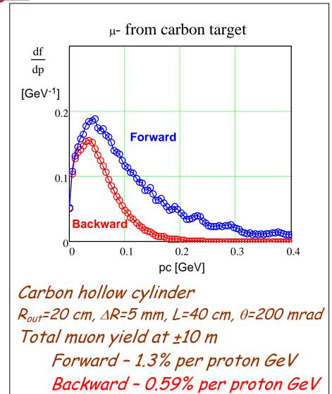
Yield per 1 GeV of proton energy: pc=3 GeV/ ( $E_{kin}=2.2$  GeV),  $\sigma_x = \sigma_y = 1$  mm - parallel beam, proton multiple scattering unaccounted
