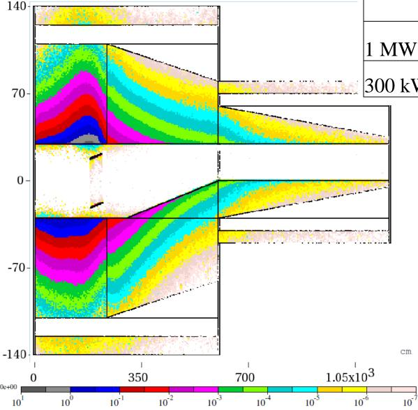
Transition from 25 kW of  $\mu$ -to-e to 1 MW increases the shield radius from ~80 cm 110 cm => B =  $5 \text{ T} \rightarrow 3 \text{ T}$  for the same stored energy
