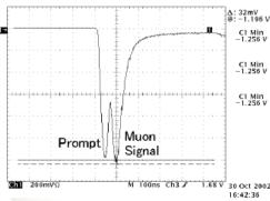
Prompt and muon signal observed at oscilloscope
