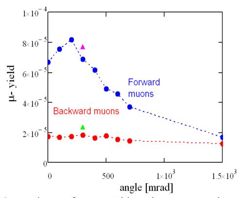
Dependence of muon yield on the target angle relative to magnetic field for carbon target into the following phase space:  $\varepsilon_x = \varepsilon_y = 1$  cm,  $\Delta p/p = \pm 15\%$ ,  $p_{prot} = 3$  GeV/c,  $(E_{kin} = 2.21$  GeV) Optimal momenta are: 100 MeV/c for backward and 200 MeV/c for forward muons
