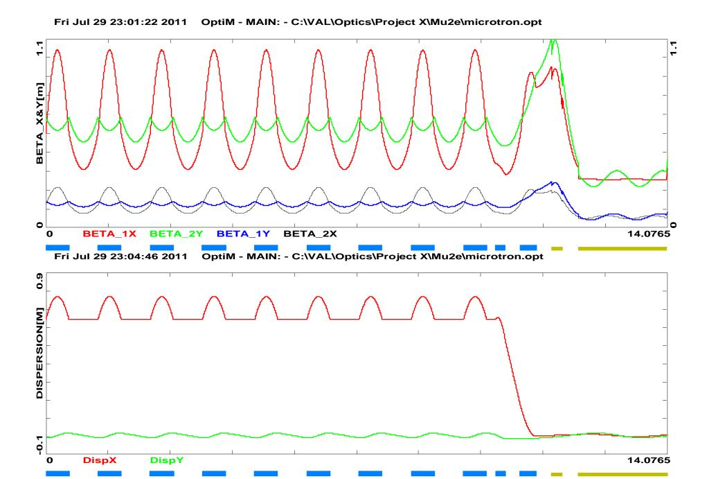
4D beta-functions (top) and dispersions (bottom) for helix and match to the detector solenoid
