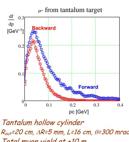
$R_{out}$ =20 cm,  $\Delta R$ =5 mm, L=16 cm,  $\theta$ =300 mrad Total muon yield at ±10 m Forward - 1.4% per proton GeV
