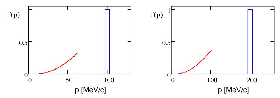
Degrading of the rectangular distribution with ±3% momentum spread
