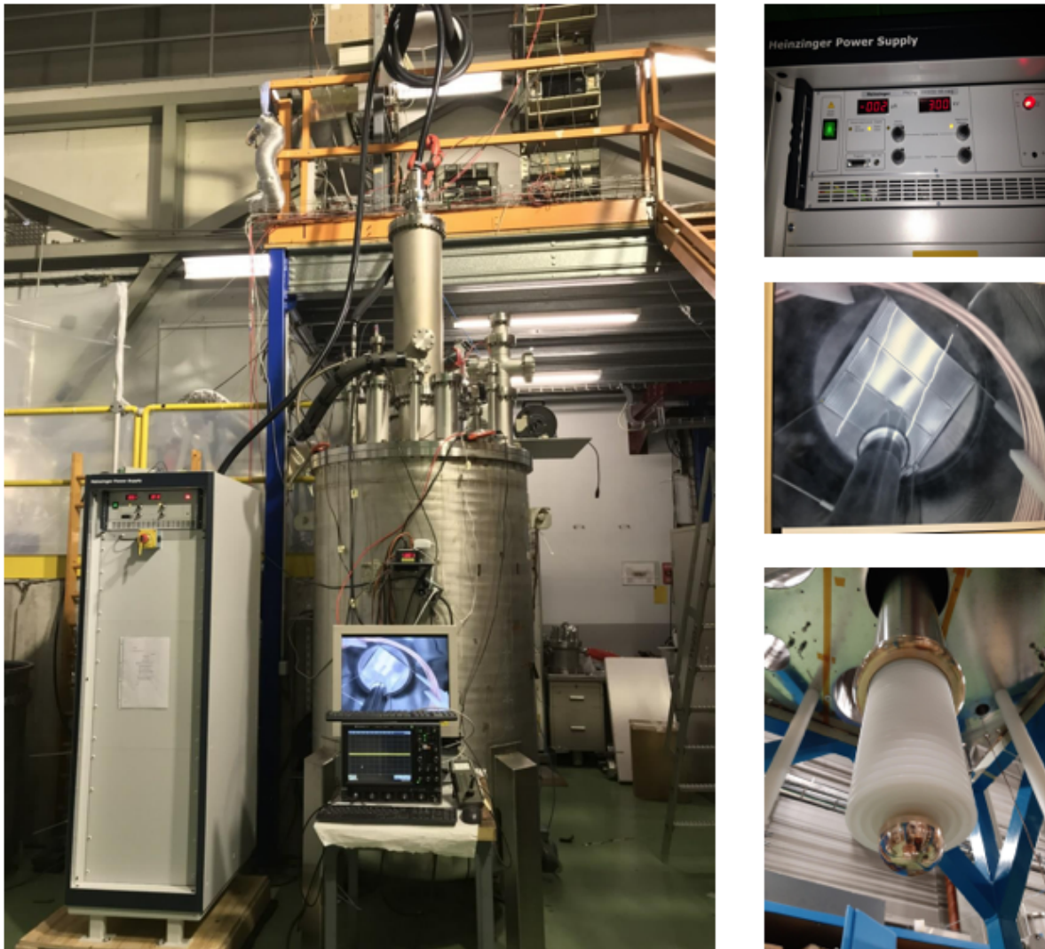
Figure 8.16: Left: test stand of the HV feedthrough. Right: details of the HVPS, the cryo-camera view and the new HVFT semi-spherical tip specifically mounted for the HVFT test.
