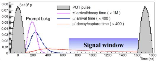
This beam structure can be realized with delivery ring manipulation for slow (resonant) extraction
