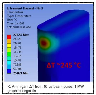
Rapid thermal expansion of material surrounded by cooler material creates a sudden localized area of high compressive stress
