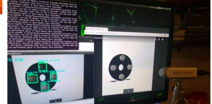
Work underway on unique and cheap robot for accelerator facility: combine computer vision and ML to identify and locate objects by UIC senior students robotics project
