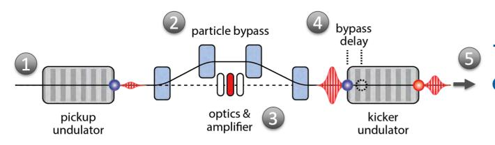
10<sup>3</sup> – 10<sup>4</sup> increase in cooling rate with OSC over SC (~10s of THz BW vs few GHz)
