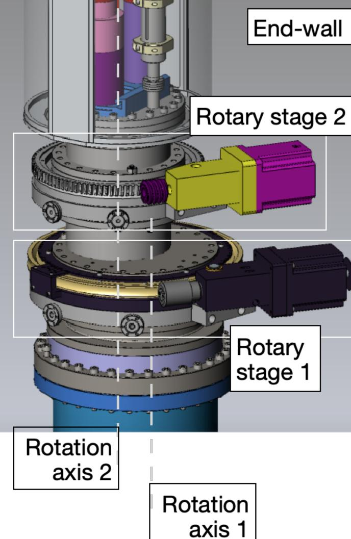
Two periscope designs to maximize coverage of the detector
