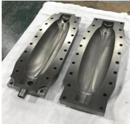
New cavity shape optimized for low flux losses
