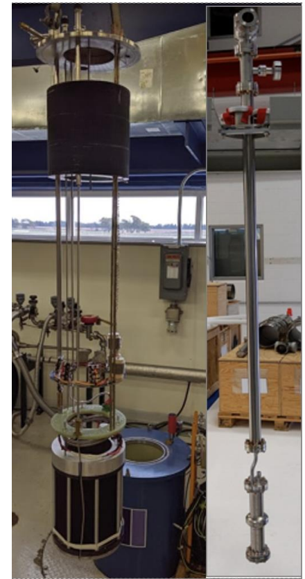
6 T solenoid (left) and \text{Nb}_3\text{Sn} cavity insert (right) at Fermilab high field magnet test facility
