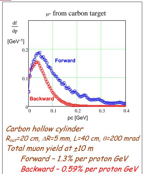
Yield per 1 GeV of proton energy: pc=3 GeV/ ( $E_{kin}=2.2$  GeV), $\sigma_x = \sigma_y = 1 \text{ mm} - parallel beam, proton multiple scattering unaccountedSmall difference between forward and backward muons for Pc<50 MeV</td>For pc<120 MeV a weak dependence on <math>E_{kin_prot}$  for  $E_{kin_prot} \in [1, 8]$  GeV/cMuon Task Force, Valeri Lebedev
