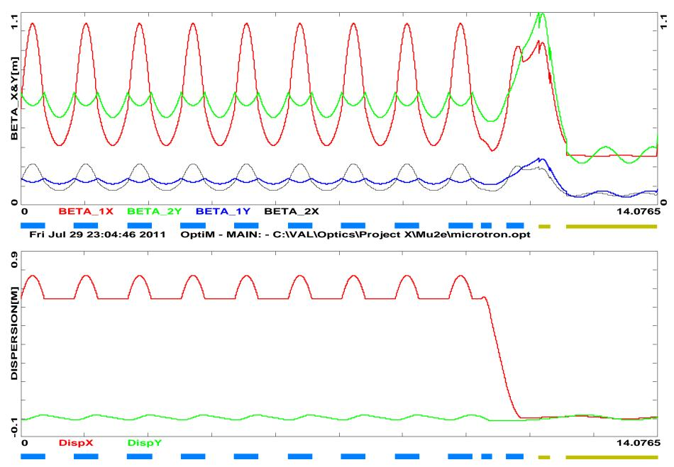
4D beta-functions (top) and dispersions (bottom) for helix and match to the detector solenoid
