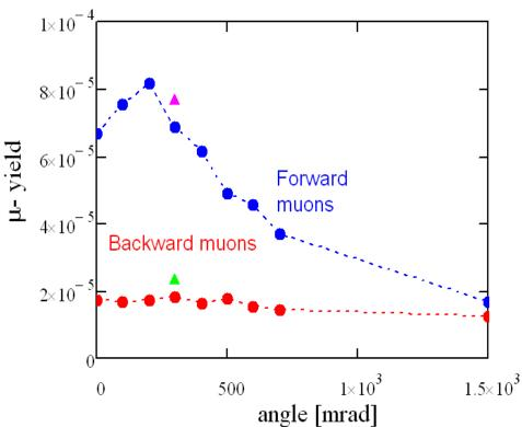
Dependence of muon yield on the target angle relative to magnetic field for carbon target into the following phase space:  $\varepsilon_x = \varepsilon_y = 1 \text{ cm}$ ,  $\Delta p/p = \pm 15\%$ ,  $p_{prot} = 3 \text{ GeV/c}$ ,  $(E_{kin} = 2.21 \text{ GeV})$ Optimal momenta are: 100 MeV/c for backward and 200 MeV/c for forward muons Triangles show results for tantalum target
