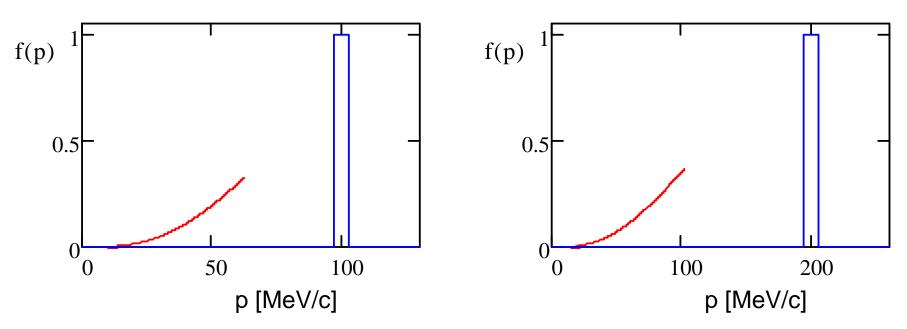
Degrading of the rectangular distribution with ±3% momentum spread The ionization cooling graded with energy looks even more exotic
