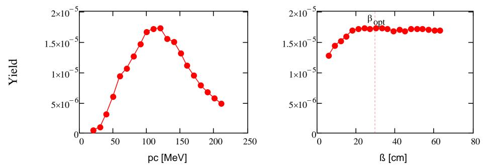
Graphite cylind. target, backward muons,  $p_{prot}=2 \text{ GeV/c}$ ,  $\varepsilon_x=\varepsilon_y=1 \text{ cm}$ ,  $\Delta p/p=\pm0.15$ ,  $\theta=200 \text{ mrad}$ , B=2.5TFor small emittance the dependence of muon yield on the  $\beta$ -function is weak Strong suppression of small energy muons (pc<50 MeV) by deceleration in medium
