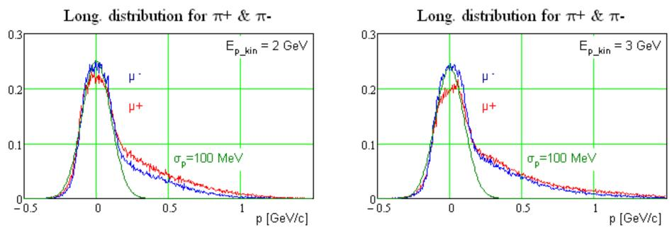
Pion longitudinal distribution function  $(df/dp_{||})/E_{p_{kin}} [c/GeV^2]$ Target - nickel cylinder, L=10 cm, r=0.4 cm; no magnetic field Total production per unit energy of incoming protons
