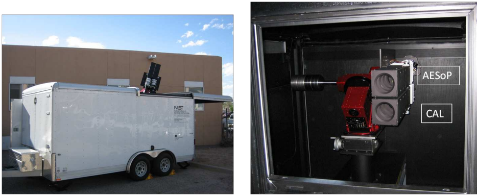
Figure 2. The picture to the left shows AESoP and CAL in the newly delivered mobile observatory with the roof open and the instruments fully elevated. The image on the right shows AESoP and CAL in their lowered calibration position looking down their baffles.
