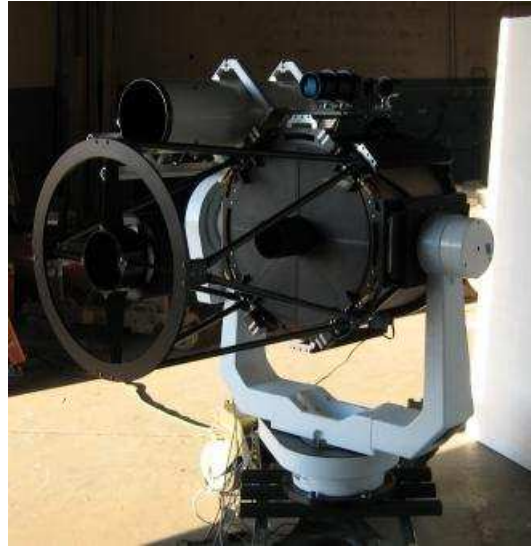
Figure 4. An image of FLAME from an assembly test is shown with one transmitter (the white 200mm telescope in the upper left) and one 75mm short range receiver (small black tube on top) attached.
